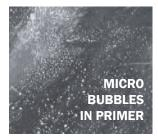
Apply the primer thin enough to minimize the formation of "micro bubbles". The primer will dry to a dull black finish. Expected drying time on a dry, sunny 70°F day could be 10 to 15 minutes.
